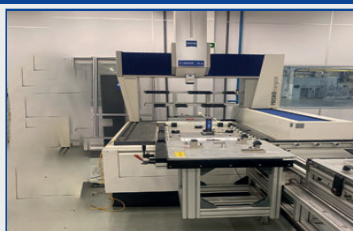
TRIDIMENSIONAL ZEISS PRISMO NAVIGATOR
